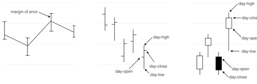
Figure 6 - Different techniques to incorporate range information, from left to right: error bars, envelopes and candlesticks. The examples are typical for use in financial market analysis.
